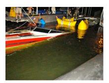
The owner was running the boat across a lake when a lower unit U joint let go and shredded the bellows seal, sinking the boat.
